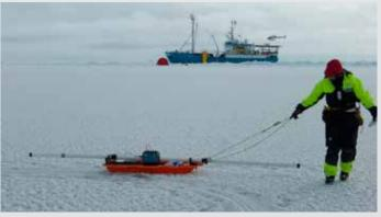
Sea ice thickness measurements are done along transects using an electromagnetic technique. Here, surveys were made during the N-ICE2015 expedition, where the research vessel Lance was frozen into drifting sea ice north of Svalbard. Results will be merged with information from helicopter surveys and remote sensing imagery, and parts of this are also used within CIRFA. Photo: Sebastian Gerland, Norwegian Polar Institute.
