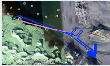
Scout flight for mapping sea ice and glaciers. This figure shows the the flight path in Kongsfjorden, Svalbard. An automatic algorithm has been developed for fast detection and size estimation of icebergs/growlers. Work is ongoing on coupling of autopilot metadata and videostreams to achieve accurate geolocation information in near real time.
