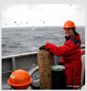
Satellite tracked drifting buoys. The spherical orange drifter is an iSphere and the cardboard cylinder contains a CODE type drifter of the same type as was deployed in summer 2015. From the 2013 Eni/NOFO HF radar experiment. (Courtesy K.H. Christensen)
