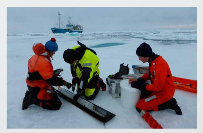
Physical properties of sea ice are crucial to understanding the state of the ice. They also affect remote sensing imagery. Here, the temperature-depth profile of the ice is measured on a newly-drilled ice core in Fram Strait, the region between Greenland and Svalbard. The Norwegian Polar Institute runs annual cruises to Fram Strait with its research vessel Lance. Photo: Sebastian Gerland, Norwegian Polar Institute
